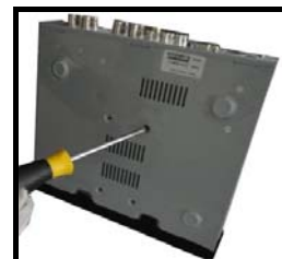
3. Fasten hard disk mounting screws.
